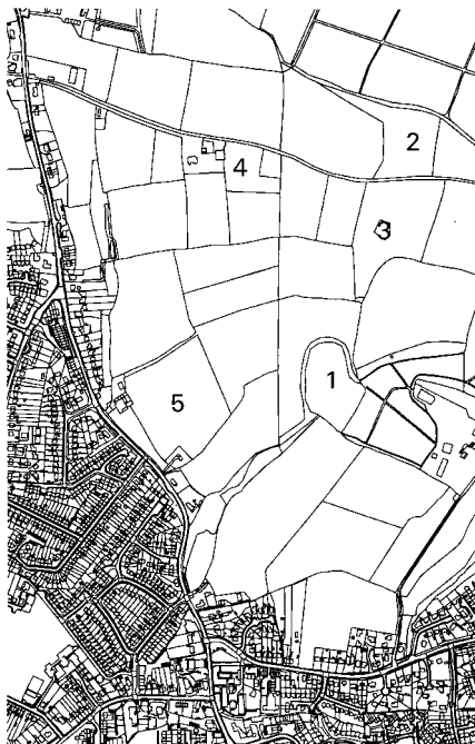
Figure 1. OS simulated DNF data showing altered features as follows: (1) Added curved boundary (double line), (2) Added curved boundary (single line), (3) Added enclosed polygon, (4) Altered land cover class and (5) removed field boundary (existed previously where the 5 is placed presently).
